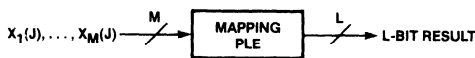
Figure 1. Mapping the j th Bit from Each of the x i 's to An L-bit Result
